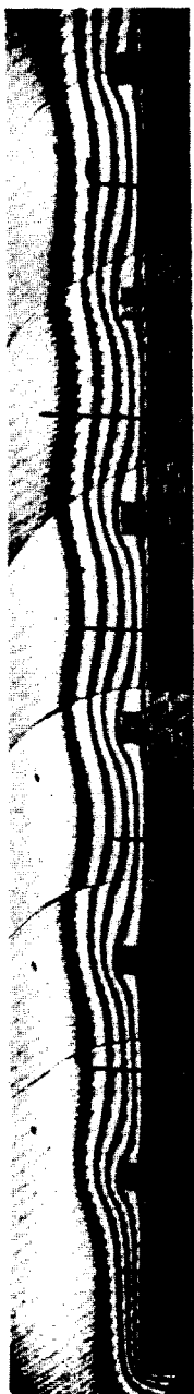
FIG. 12. Composite interferogram of a ribbed plate with p/s = 8:1 and p/q = 8:1 (low conductivity ribs).
